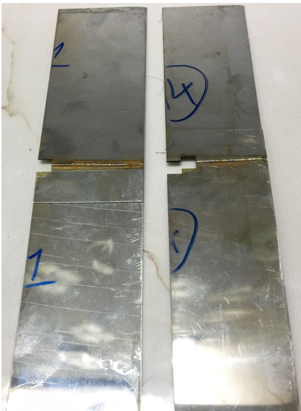
Fig. 4. Close view of two typical welded samples in lap joint configuration
