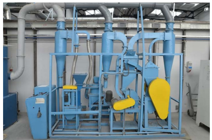
Fig. 1. Mechanical reclamation station installed at the Foundry Research Institute
