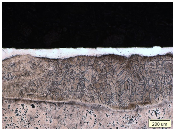
Fig. 2. Austenitic stainless steel 316L alloyed with FeCr, laser beam power 2.1 kW, powder feed directly to the molten metal pool
