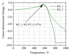
Fig. 6. Dilatometric curves for moulding sand M2
