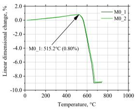
Fig. 4. Dilatometric curves for moulding sand M0
