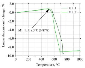
Fig. 5. Dilatometric curves for moulding sand M1
