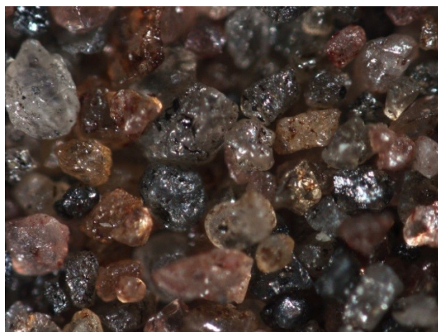
Fig. 3. Micrograph of foundry 4 sand as received
