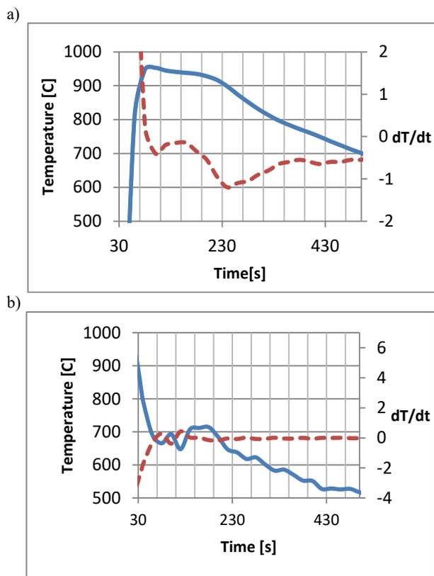
Fig. 2. MO59 brass cooling curves a) temperature course [ $^{\circ}\text{C}$ ] over time, b) cooling curve of the liquid alloy free surface - pyrometer measurement (dotted line)
