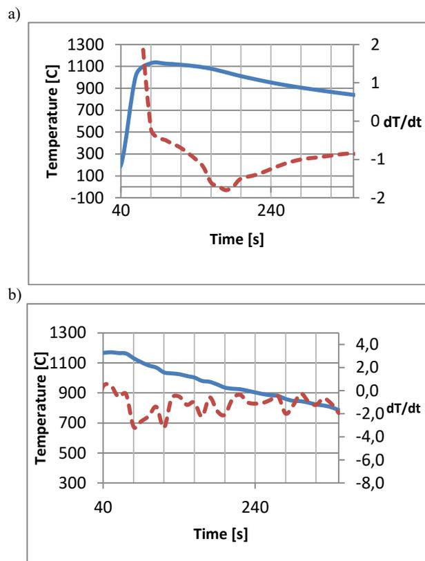
Fig. 3. M95 brass cooling curves a) temperature course [ $^{\circ}\text{C}$ ] over time, b) cooling curve of the liquid alloy free surface - pyrometer measurement (dotted line)
