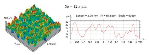
Fig. 3. Surface texture of Inconel 718 after the EDM ( $I = 13.5 \text{ A}, t_{\text{on}} = 145 \text{ }\mu\text{s}$ )
