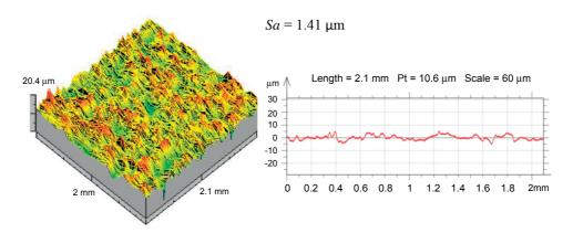
Fig. 4. Surface texture of Inconel 718 after EDM ( $I = 1.7 \text{ A}, t_{\text{on}} = 78 \text{ }\mu\text{s}$ )
