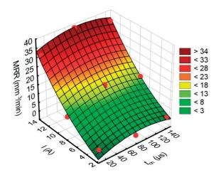
Fig. 8. Estimated response surface for material removal rate
