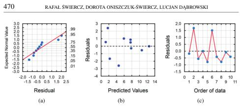
Fig. 5. Plots for the check model of the arithmetic mean of the deviations from the mean *Sa*: (a) the normal plot of residuals, (b) the residuals versus the predicted values, and (c) theresiduals versus the order of the data
