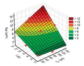
Fig. 6. Estimated response surface for the arithmetic mean of the deviations from the mean *Sa*
