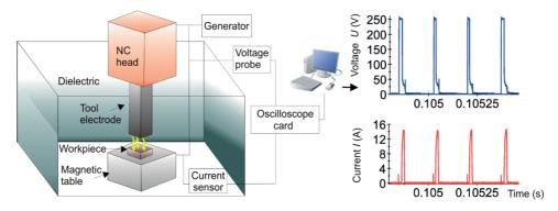
Fig. 1. Scheme of the EDM process, with the measured current-voltage waveforms for the following settings U = 25 V, I = 14 A,  $t_{on} = 10 \ \mu s$ ,  $t_{off} = 150 \ \mu s$
