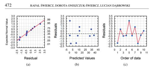
Fig. 7. Plots for the check model of the *MRR* (a) the normal plot of residuals, (b) the residuals versus the predicted values and (c) the residuals versus the order of the data
