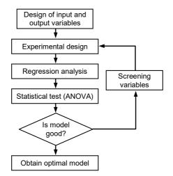
Fig. 2. The procedure of the model development with the Response Surface Methodology
