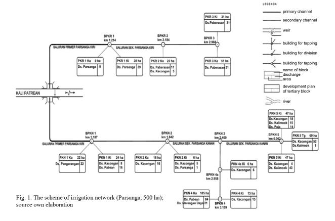
consist of 8 villages. The irrigation area is 500 ha and the scheme of irrigation network is presented as in the Figure 1.
