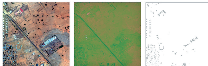
Fig. 19. Semantic segmentation results using multi-spectral U-Net architecture. Left: RGB satellite input image. Middle: Infrared satellite input image. Right: Semantic segmentation results for buildings
