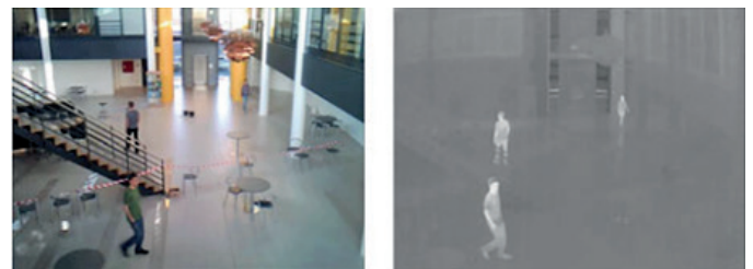
Fig. 1. Visible and thermal image of the same scene [1]
