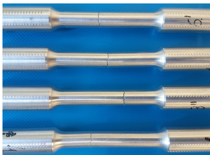
Fig. 10. Samples after a tensile test
