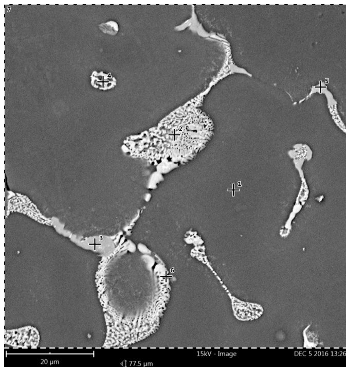
Fig. 6. Structure of the ingot cast with an average speed of 100 mm/min; cross-section (SEM)
