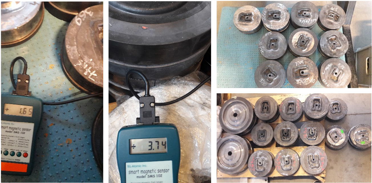
Fig. 11. Exemplary tools and selectet results of the residual magnetic field analysis
