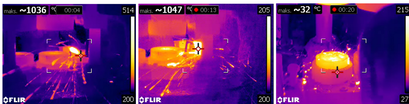
Fig. 9. Visible scale chipping from the forging material and lying on the lower upset dies
