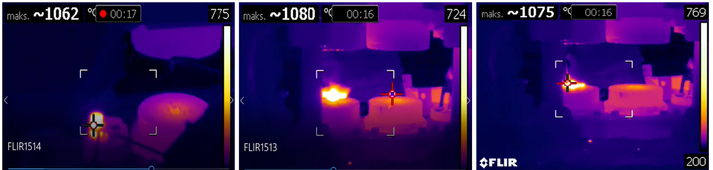
Fig. 4. Stand for forging “yoke” forging, temperature measurement after flattening operations, initial and finishing forging – temperature of the forging
