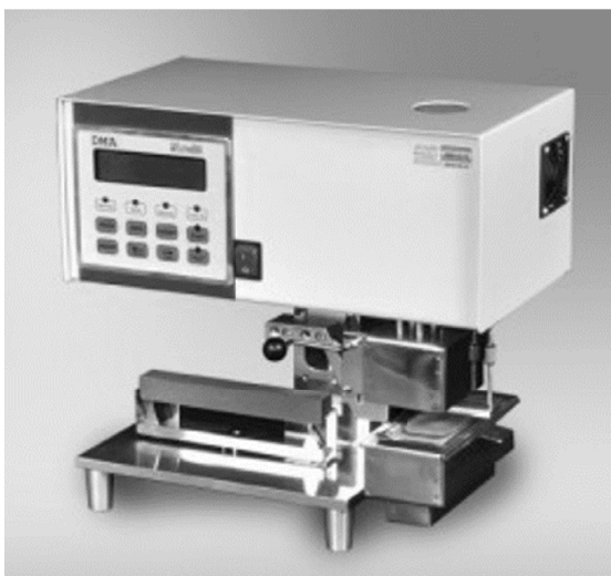
Fig. 2. Universal apparatus for studying hot-distortion phenomena and bending strength, produced by Multiserw-Morek Company [10]
