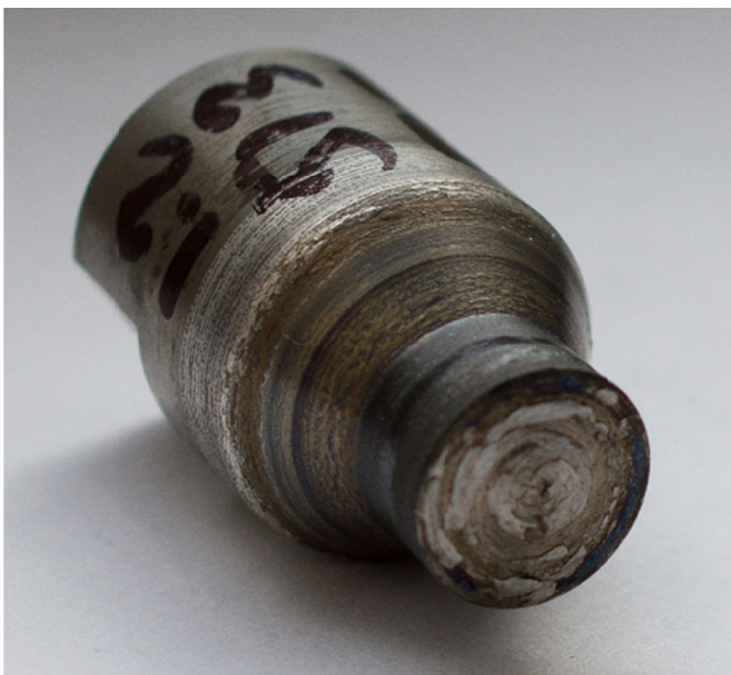
Fig. 9. Working surface of worn FSW tool (tool material: W-25Re)
