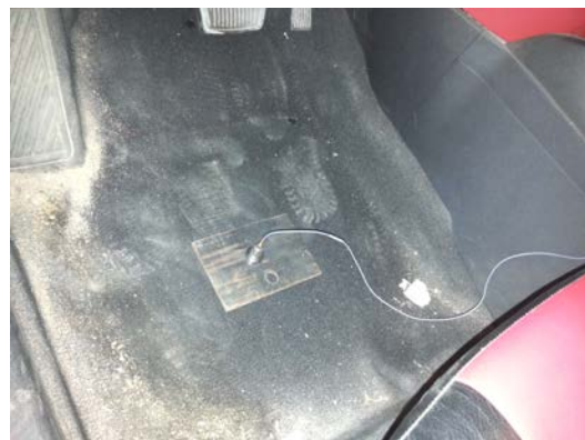
Fig. 2. Accelerometer positions on vehicle floor.
