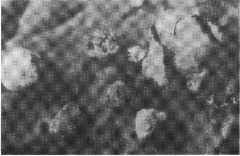
Fig. 8. Phosphatization of the sand fraction in the profile No. 6 depth 5—45 cm Clay pseudomorphs after fragments of the rock surrounded by hard coat of phosphates. Magnification 40x
