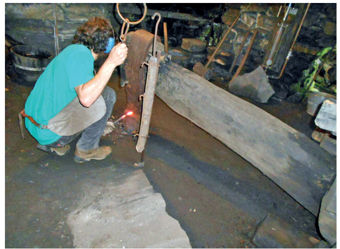
Fig. 5. Forging process by blows of the drop hammer
