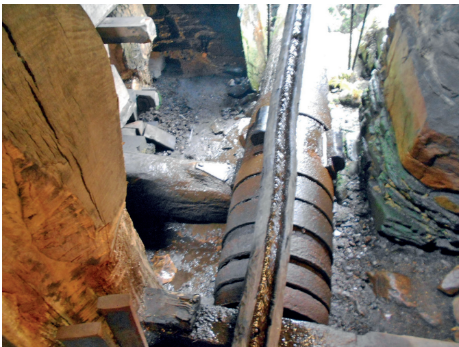
Fig. 4. Detail of the teeth forming the cams ( malobreiros ) and the cooling channel of the transmission shaft supports
