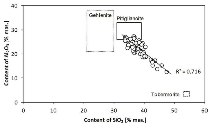
Fig. 9. Participation of SiO<sub>2</sub> and Al<sub>2</sub>O<sub>3</sub> in the studied grains against the background of the theoretical differentiation of the content of these components in tobermorite, pitiglianoite and gehlenite
