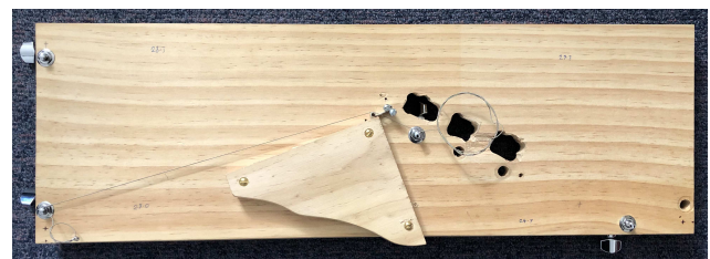
Fig. 4. Photograph of the one-string guitar modified to have seven possible tuning peg positions. Screws were used to secure the saddle in place, along with an additional piece of wood underneath to prevent the saddle moving when a string under high tension is passed across.
