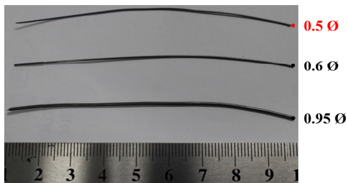
Fig 4. Manufacturing of tantalum wires by drawing
