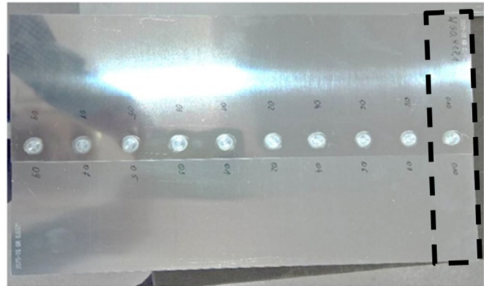
Fig. 1. View of the fabricated joints – sample with 10 welds with pointed single sample (210 × 30 mm)
