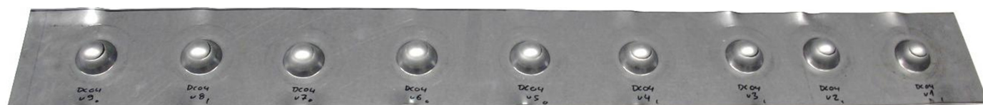
Fig 2. Sheet strip with cups made during tests
