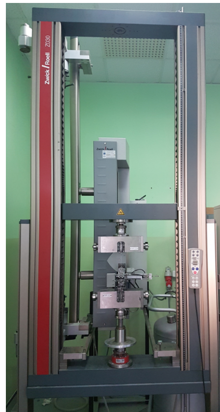
Fig. 10. ZWICK Z030 testing machine used in the laboratory research
