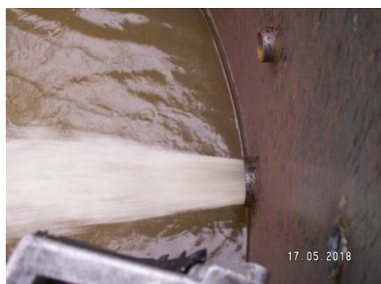
Photo 3. The mixing system in the reactor – pressing of the inert agent during the tightness test (phot. G. Walowski)
