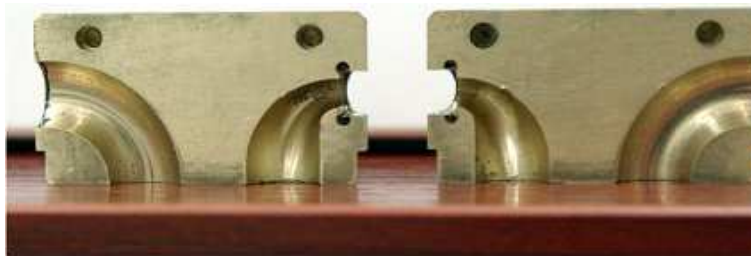
Figure 8: Photo showing elements of the bucket head of the Roto-Jet pump [26].
