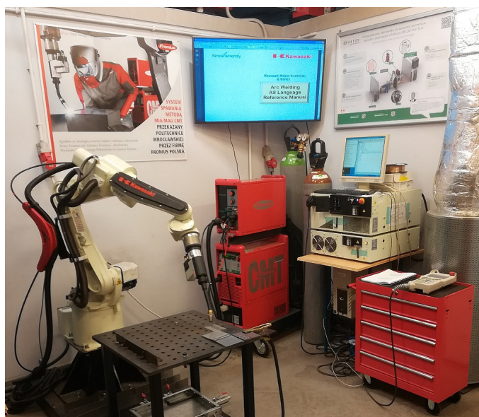
Fig. 15. Robotic welding station for CMT process assembled of Kawasaki BA006 welding robot and Fronius TransPuls Synergic 3200 welder with equipment
