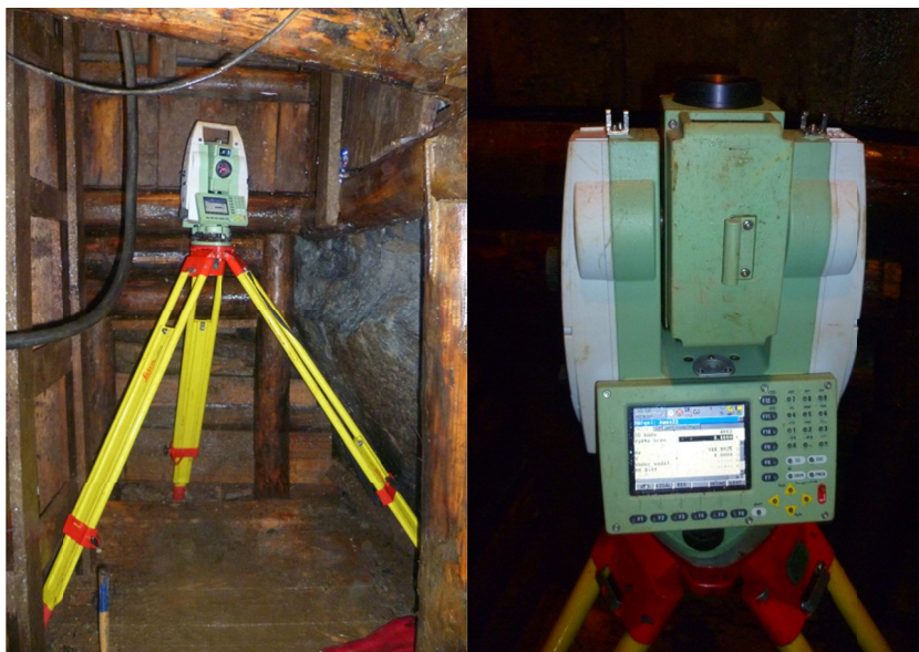
Fig. 8. Total station on the shaft bottom with zenith measure
