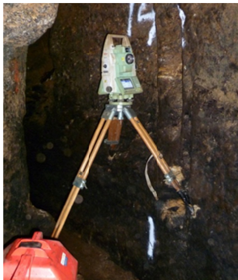
Fig. 5. Example of tripod legs installed in pockets cut in the adit wall
