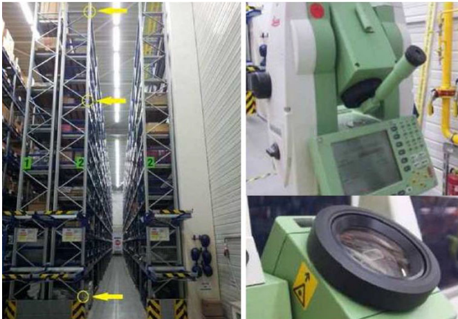
Fig. 7. The layout of detailed survey points and the diagonal eyepiece
