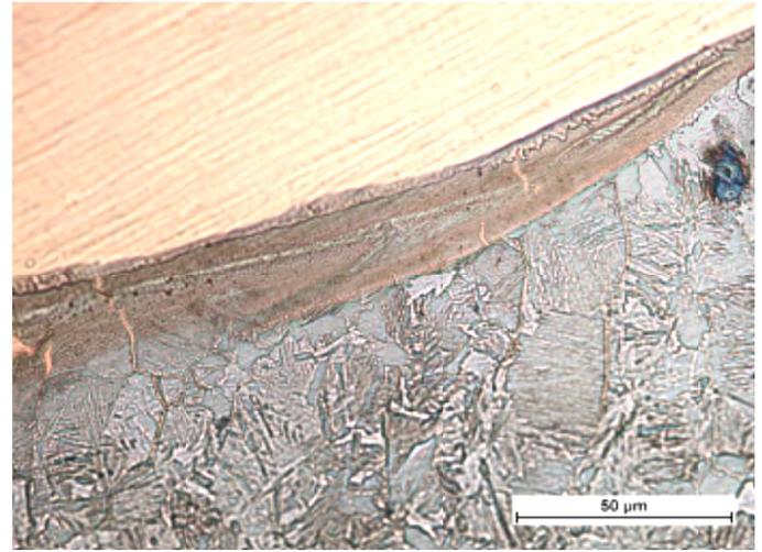
Fig. 7. View of cracks filled with liquid solder
