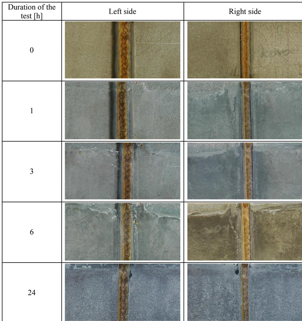
Fig. 11. TIG brazed welded butt joint Z7 after the electrochemical corrosion resistance test based on the galvanostatic method
