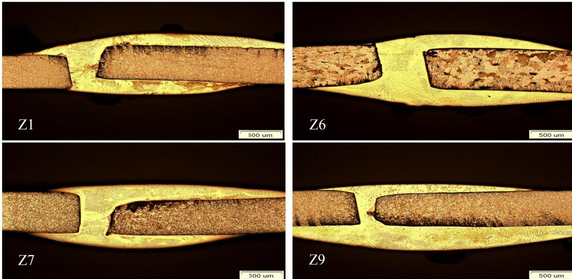
Fig. 4. Macrostructure of the TIG braze welded butt joints made using the CuSi3Mn1 braze; etchant: Nital + FeCl<sub>3</sub>
