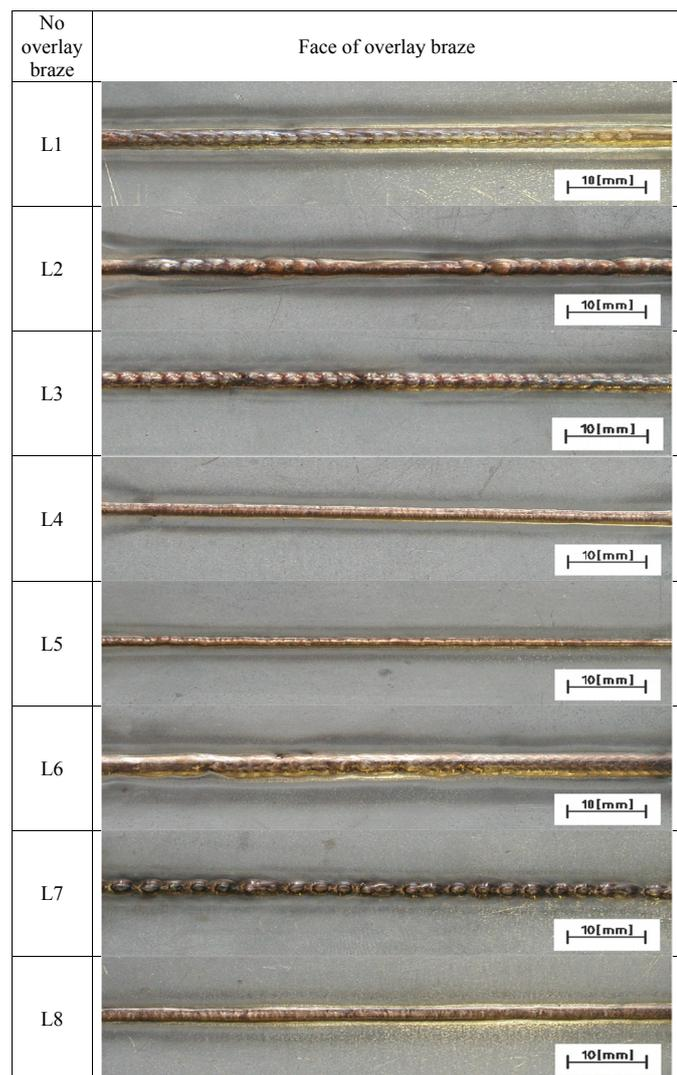
Fig. 2. Face of overlay brazes made using the TIG method
