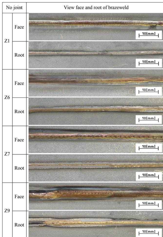
Fig. 3. Brazewelds made using the TIG method
