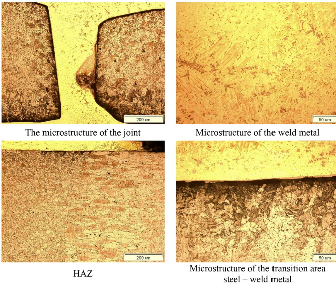
Fig. 5. Microstructure of the butt joint – specimen Z9
