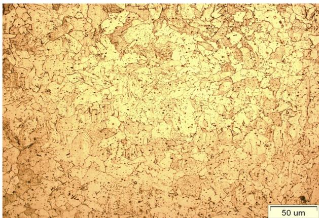
Fig. 1. Ferritic microstructure of steel DC04 (EN 10130)
