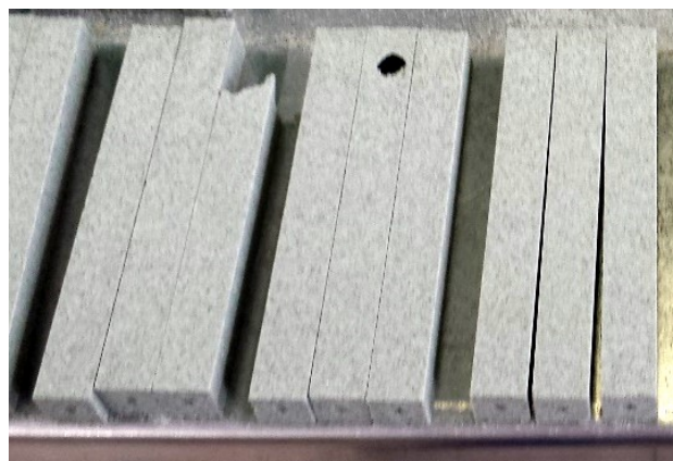
Fig. 4. Example of dimensionally - shaped defects in made from olivine SSBS cores caused by inadequate adjustment of the LUT/c/CO 2 /An device's operating parameters
