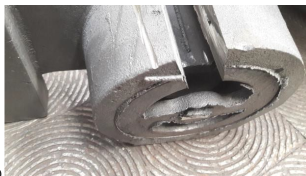
Fig. 7. Casting tree incl. Flow off tanks (a) and cut off position (b)
