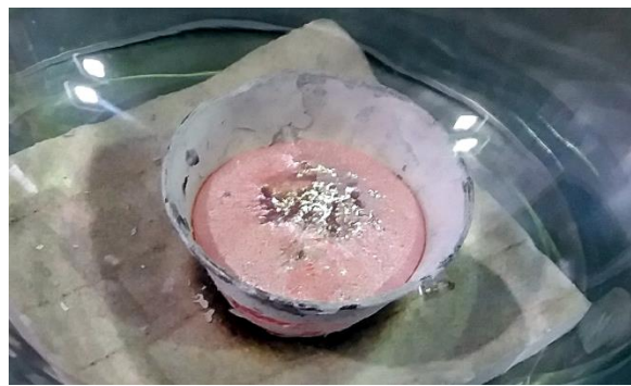
Fig. 3. RPT sample inside the vacuum chamber with bubbling hydrogen on the surface of the aluminium taken from the metal bath at 800°C
