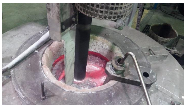
Fig. 2. Rotary degasser in the medium volume furnace
