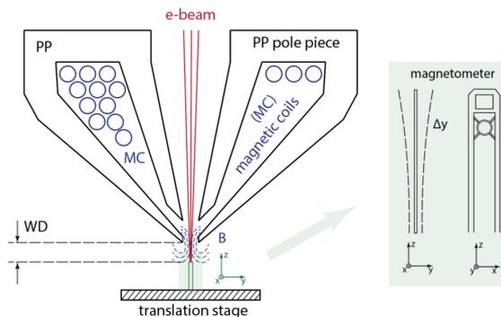
Fig. 1. A schematic of the immersion lens and the magnetic field area inside the SEM/FIB vacuum chamber (not in scale).
