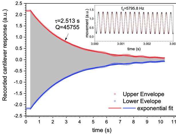
Fig. 5. The ring-down technique for quality factor evaluation: the upper and lower envelopes of the micro-cantilever response fitted with the exponential decay function (main plot) and the resonance frequency measurement by sine fitting to a section of the response (inset).
