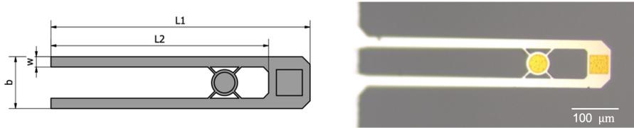
Fig. 3. A micro-cantilever magnetometer used for determination of the magnetic field under the e-beam column: a schematic (left) and a real view (right); dimensions:  $L_1 = 515 \mu\text{m}$ ;  $L_2 = 465 \mu\text{m}$ ;  $b = 100 \mu\text{m}$ ;  $w = 20 \mu\text{m}$ .
