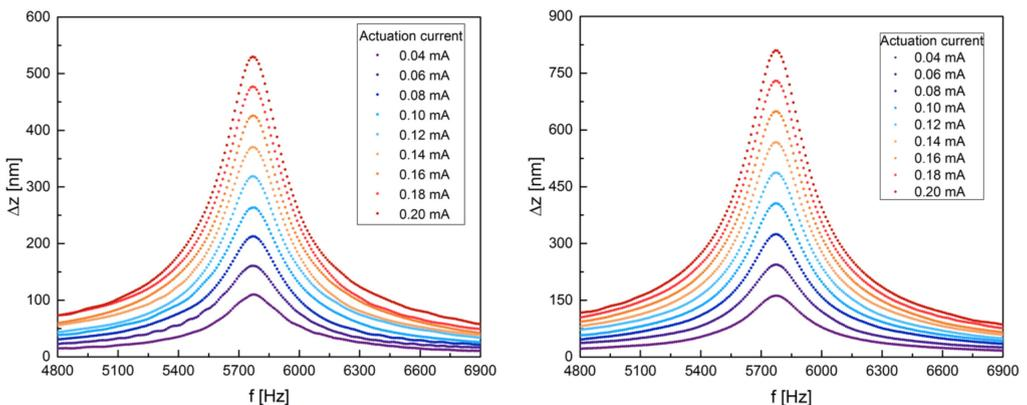
Fig. 4. MetMolMEMS resonant vibration amplitude: the lower mirror read-out (left), detection of the upper mirror read-out; measurement done with the SIOS vibrometer (right).
