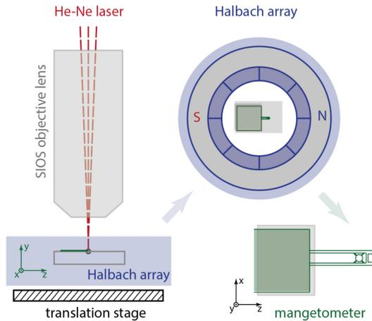
Fig. 2. A precise setup for the micro-cantilever magnetometer parametrization calibration: Halbach array under SIOS vibrometer for the deflection measurement.
