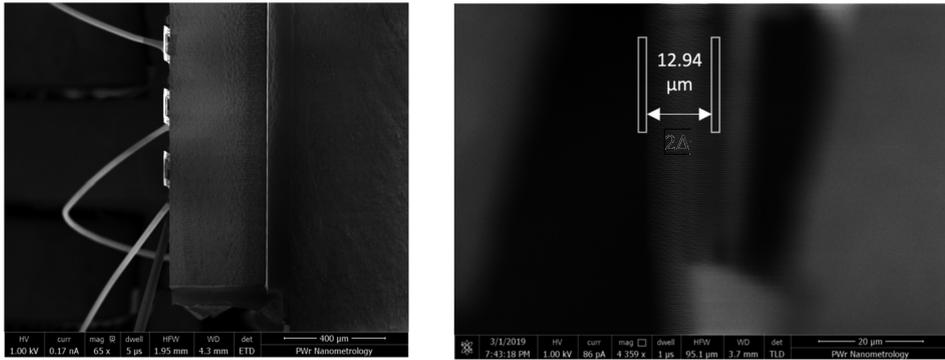
Fig. 6. The micro-cantilever magnetometer in FIB/SEM chamber: a top view from the adjustment process (left), SEM vibrometry – the measured displacement (right).
