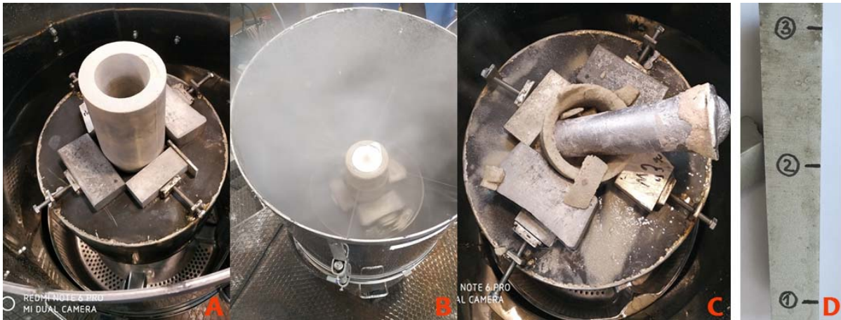
Fig. 4. The experimental cast in the modified ablation casting: A) sand mould, B) ablation process, water erosion, C) ready casting, D) cut casting with marked measurement levels
