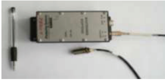
Fig.4. Kaman system KD2300 for small deformation measurement
