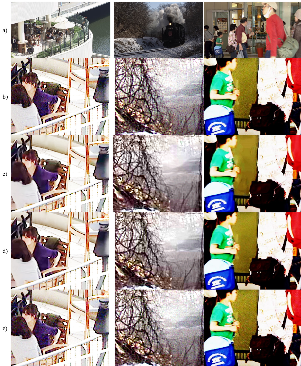
Fig. 10. Examples of images from sequences “BQt terrace” (left), “Steam Locomotive” (middle) and “BQMall” (right). a) Original frame, b) enlarged and contrast-enhanced original fragment. Encoded videos (rate R4): c) A. Anchor, d) B. Noise Reduction, e) C. Proposal.
