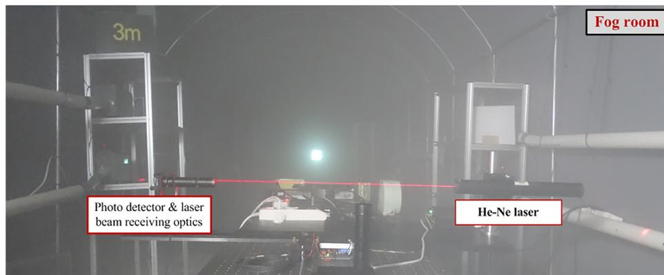
**Fig. 6.** A laser beam attenuation measurement of the He-Ne laser in the fog room under fog spray environments.
