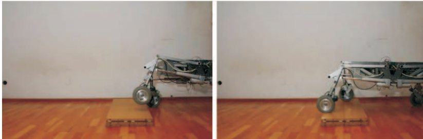
Fig. 16. Testing of walking function – obstacle in front of one wheel
