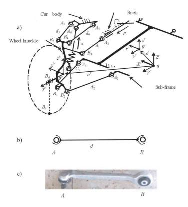
Fig. 1. a) Kinematical model of the wheel guide mechanism; b) Kinematic model of a separate link; c) View of real link of mechanism
