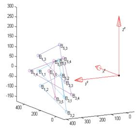
Fig. 4. The successive positions of the measured plate determined on the base of coordinate measurements with respect to the basic frame
