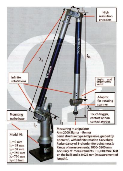
Fig. 2. View of measurement manipulator and some specifications [10]
