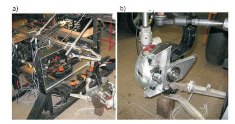
Fig. 3. a) View of 5-link suspension mechanism assembled with the base frame of the rig; b) View of the additional platform fixed to the wheel knuckle with measured points
