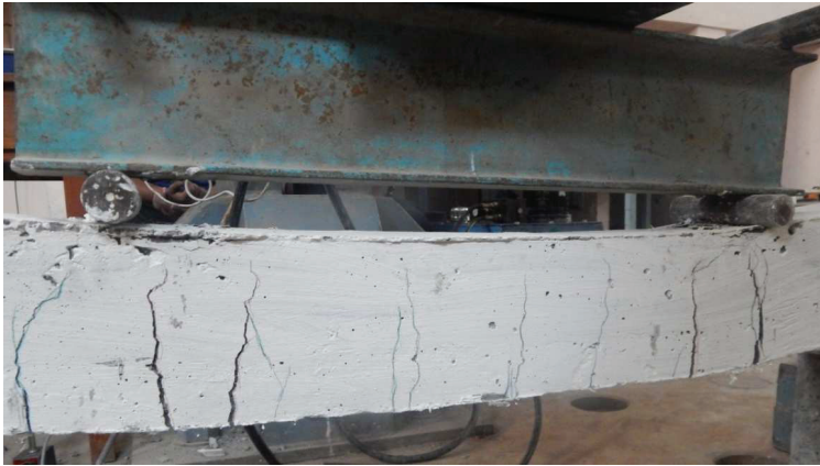
Figure 7. Typical deflection behavior of an ECC layered beam under ultimate loading
