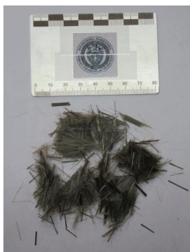
Fig. 1. Basalt-polymer fibers with a length of 12 mm
