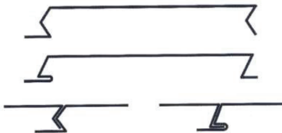
Fig. 7. Complementary interlocking planks, at the top - fitted out with chevron joint, in the middle - fitted out with clip joint, at the bottom - examples of the locked chevron and clip joints.
