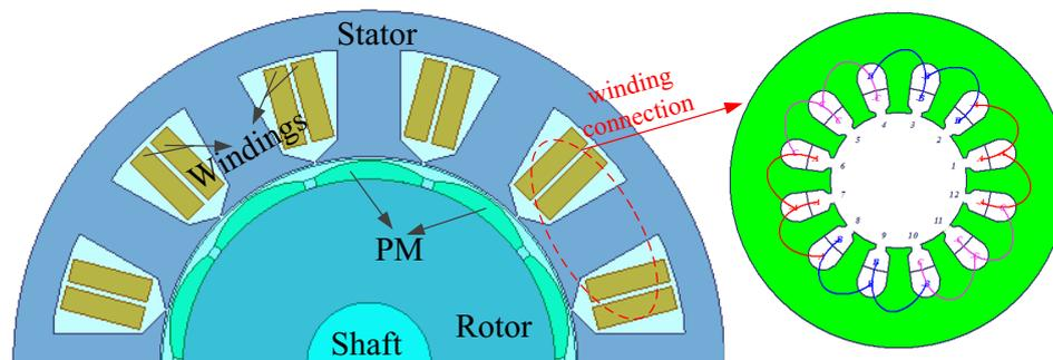
(a) The finite element model of CW-12slot
