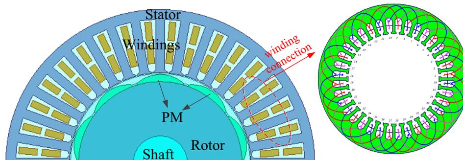
(b) The finite element model of DW-30slot
