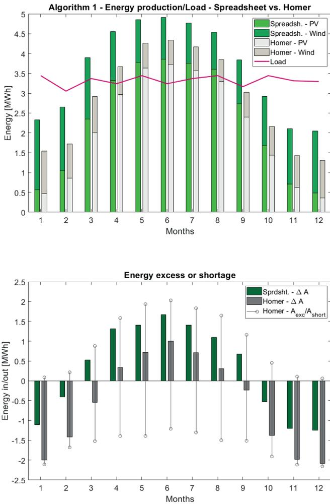
Fig. 5. Results over a year obtained from Spreadsheet and HomerPro on the basis of monthly analysis solution
