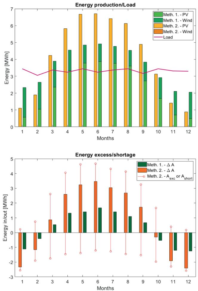
Fig. 4. Energy production and load and excess and shortage energy over a year solved with use of method 1 – monthly data, and method 2 – hourly data
