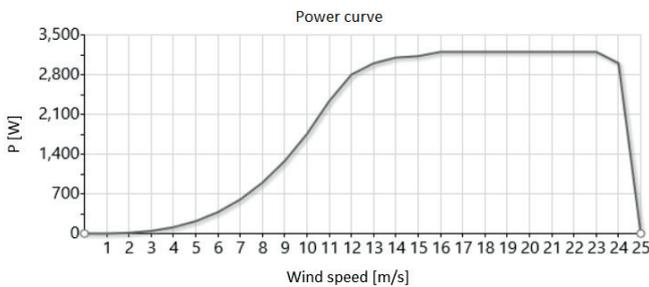
Fig. 1. Power-wind speed curve of selected wind turbine
