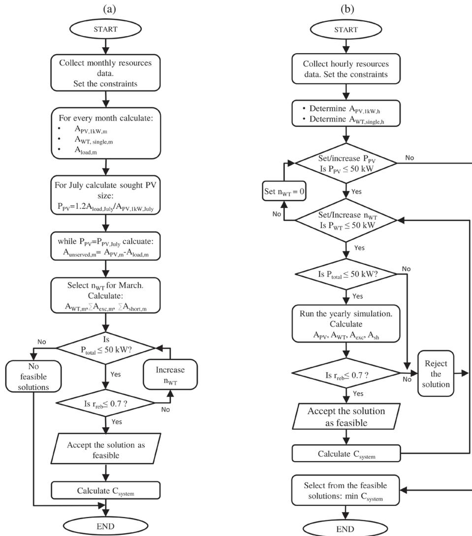
Fig. 3. The algorithm to select power of renewable sources: a) on the basis of monthly balance, b) on the basis of hourly balance
