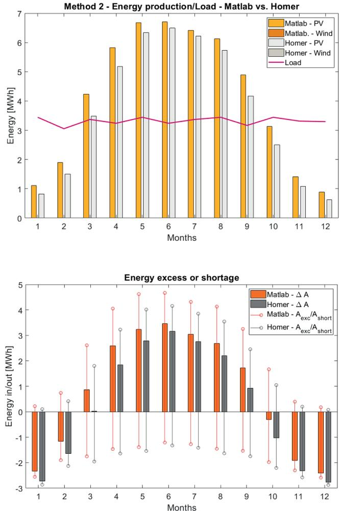
Fig. 6. Results over a year obtained from Matlab and HomerPro on the basis of hourly analysis solution
