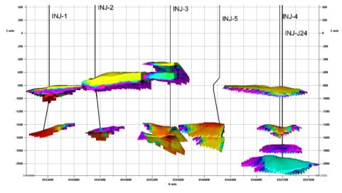
Fig. 5. CO<sub>2</sub> plume after 15 years of injection Source: [23]
