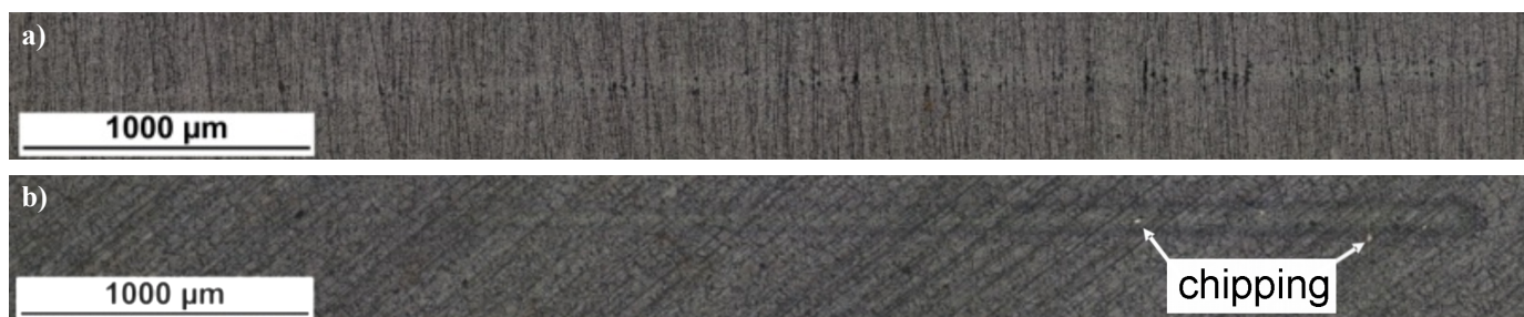
Fig. 3. Scratch images of DLC coatings produced in (a) DC and (b) pulsed glow discharge conditions on nitrided 316L steel
