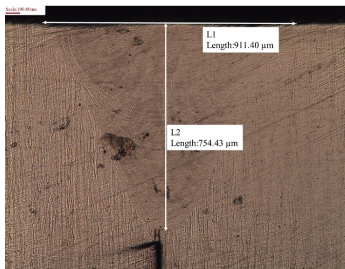
Fig. 6. Resolidified zone for case of continuous electron beam welding in cross-sectional view
