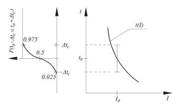
Fig. 2. Time-current characteristic of a fuse and its statistical description of uncertainty for assumed confidence level of 0.95
