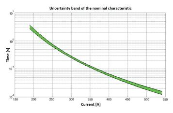
Fig. 9. Uncertainty band of the current-time characteristic calculated on the basis of the confidence ellipse, with the dark lines marking the boundary characteristics according to the further specified confidence interval of operation time
