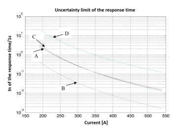
Fig. 7. Limits of uncertainty current-time characteristic of the tested fuses determined on the basis of confidence intervals of approximation parameters: A: An, max<sub>n,min</sub>; B: An, min<sub>n,min</sub>; C: An, min<sub>n,max</sub>; D: An, max<sub>n,max</sub>
