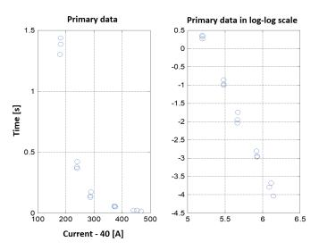
Fig. 4. Primary data - results of measurements of operating time of 15 fuses with rated current of 40 A
