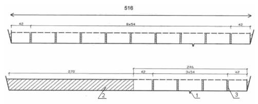
Fig. 1. A scheme of road crossing the river valley; 1 - river, 2 - embankment, 3 - piers (estacade)
