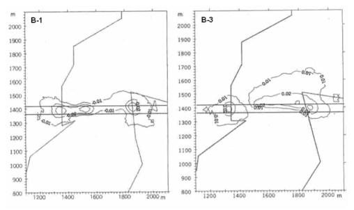
Fig. 5. Changes of groundwater tables in the valley: scenario B-1 and B-3; isolines every 0.01 m
