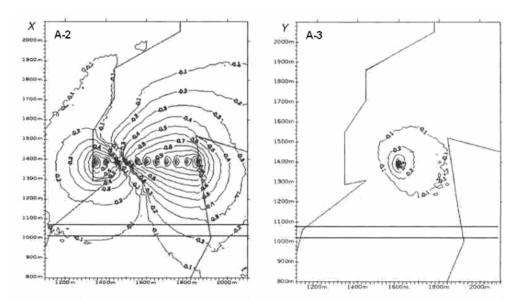
Fig. 4. Changes of groundwater tables in the valley: scenario A–2 and A–3; isolines at every 0.1 m
