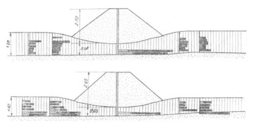
Fig. 7. The examples of cross-section of the road embankment crossing the river valley. The results of shear strength measurement
