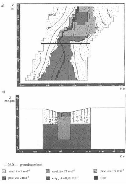
Fig. 3. The river valley; a) plan, b) cross section A – A as shown in Fig 3a
