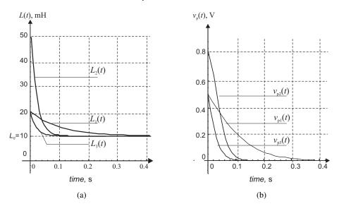
Fig. 10. Parameters variability of LTV coil: varying inductance: L(t) (a); control voltage  $v_D(t)$  (b)
