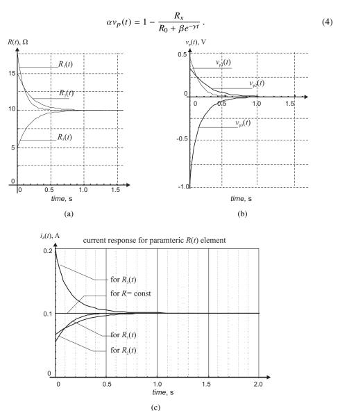
Fig. 4. Simulations for LTV resistor: varying resistance R(t) (a); control voltage  $v_p(t)$  (b); current waveforms through the parametric resistor for unit-step voltage (c)
