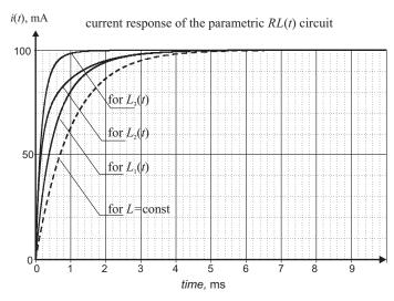
Fig. 12. Current response of RL(t) system of an LTV filter to a unit step in the case of various alterations of parameter L(t)
