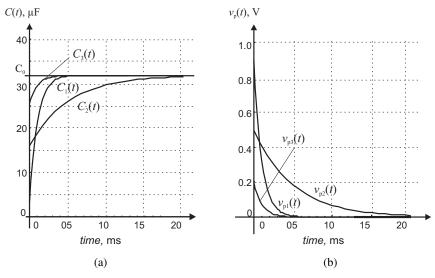
Fig. 6. Parameters variability of LTV capacitor: varying capaciance C(t) (a); control voltage  $v_D(t)$  (b)
