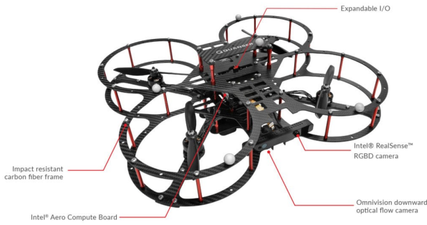
Fig. 7. Main elements of QDrone. Source: [26].
